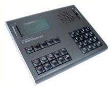
**TE10-39/3** Radio Dispatch Terminal has been designed to provide control of up to 4 Radio Base Stations at the same time. The Dispatch Terminal is equipped with push buttons for selection of Monitoring of the communication conducted on the radio channel as well as push buttons for switching the Base Station transmitter "ON" and thereby make it a part of the communications group.
